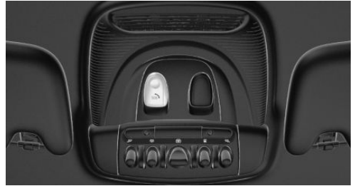
SOS button in the roofliner
